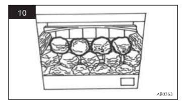
• Put the last three round coals behind the centre row and touching the back panel, Diagram 11
